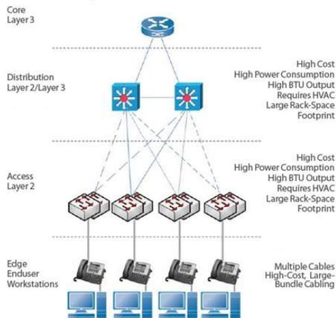
Fig 1. Typical Ethernet LAN Topology.
