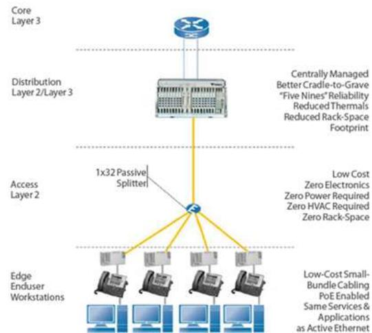
Fig 2. Passive Optical LAN Architecture
